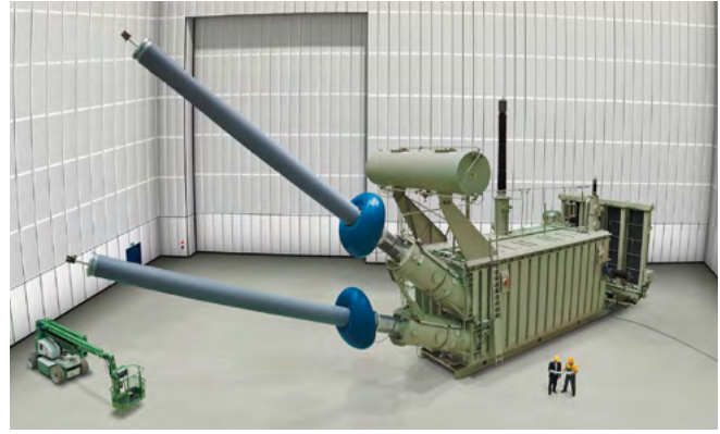
Fig. 5.10-1: Converter transformer for UHVDC bipolar transmission system \pm 800 kVDC, 6,400 MW; 2,071 km: single phase; 550 kVAC, 816 kVDC; 321 MVA; high-pulse wye system feeding
