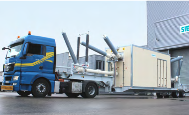
Fig. 2.4-11: 245/60-30 kV 40MVA mobile substation: High voltage switchgear trailer
