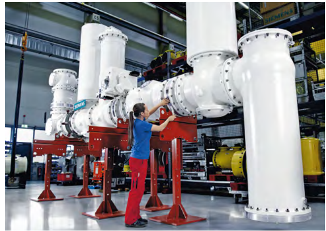
Fig. 2.2-13: 320 kV DC compact switchgear in the Siemens factory in Berlin
