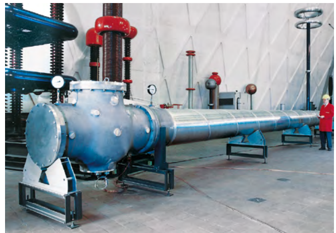
Fig. 2.2-43: Siemens lab sample for dielectric tests
