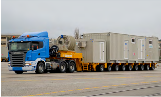
Fig. 2.4-12: 36kV/12kV 16 MVA mobile substation
