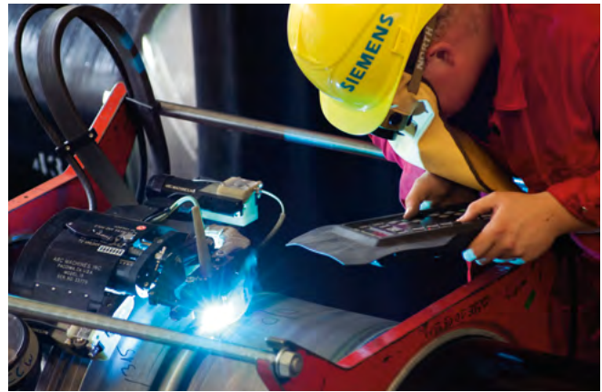
Fig. 2.2-44: Orbital welding of GIL pipes
