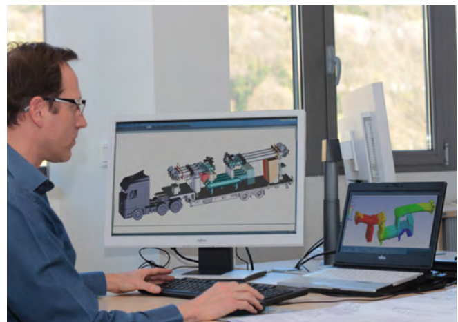
Fig. 2.4-22: Structural mechanical design for mobile substation: combined trailer & HV GIS Mechanical stress analysis during transportation
