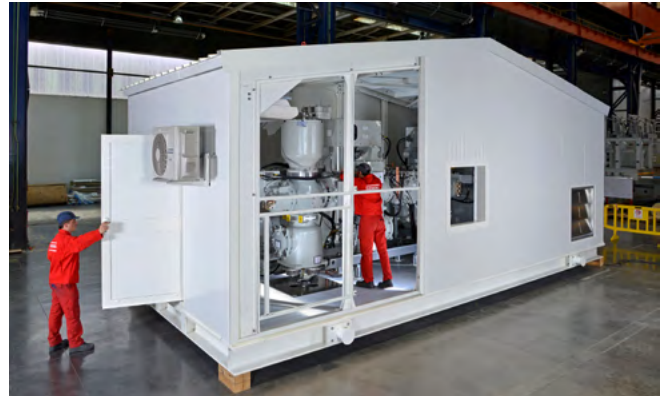
Fig. 2.4-2: High Voltage GIS E-house project for transmission substation (France)
