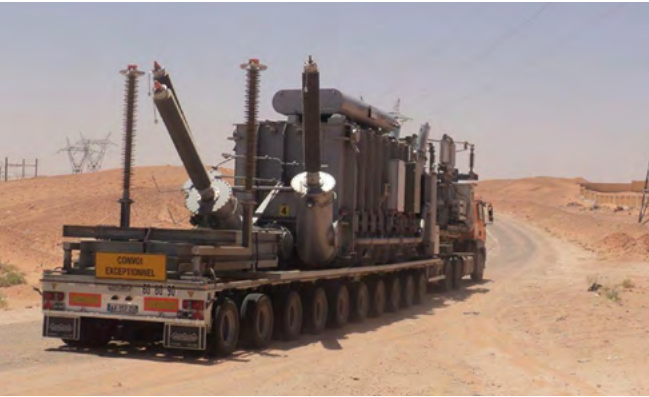
Fig. 2.4-10: 245/60-30 kV 40MVA mobile substation: Transformer trailer
