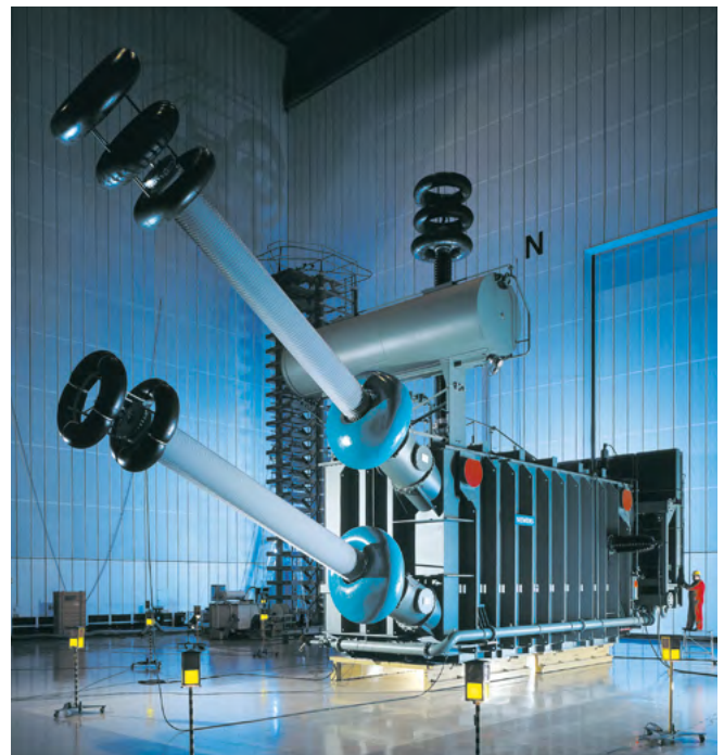
Fig. 4.2-49: Transformer bushing – 500 kV HVDC – project Three Gorges, China
