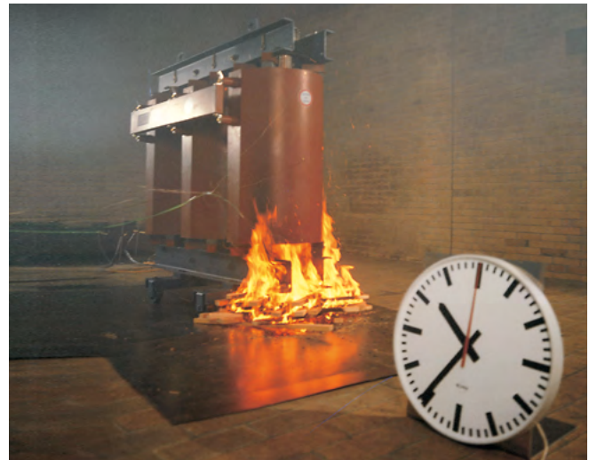
Fig. 5.11-7: Flammability test of cast-resin transformer
