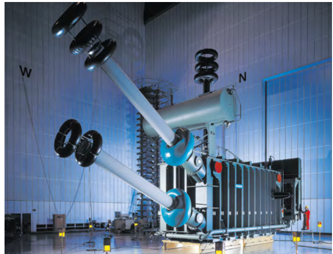
Fig. 5.10-2: Converter transformer for HVDC bipolar transmission system \pm 500 kVDC; 2,500 MW: single phase; 420 kVAC; 515 kVDC; 397 MVA; wye system (left side of figure), and delta system (right side of figure)
