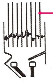
Voltage drop across each baffle extinguishes the arc
