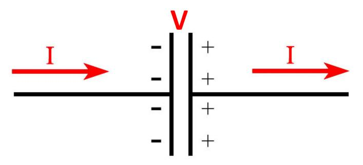
The current flows immediately to the other side, but the voltage builds across the capacitor.
