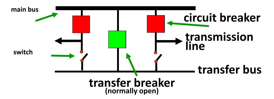
Transfer breaker & switch allows either line to remain energized while its normal breaker is out for maintenance...
