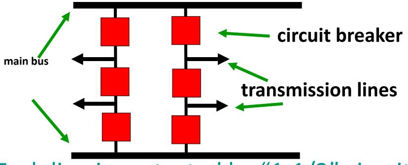
Each line is protected by "1-1/2" circuit breakers.
