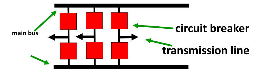
Each line is protected by two circuit breakers.
